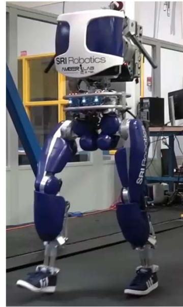
Multi-contact walking demonstrated on DURUS (Designed by SRI, 15 actuated joints, 23 degrees of freedom)
